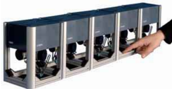
Figure 3: Microfactory concept for a desktop assembly line with 5 PocketDelta robots
